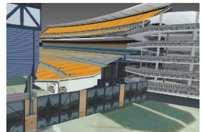
RIGHT: A model of Heinz Field was created so that a CFD analysis could be conducted using Autodesk's Project Falcon's 3D visualization capabilities. Image courtesy of Autodesk.
