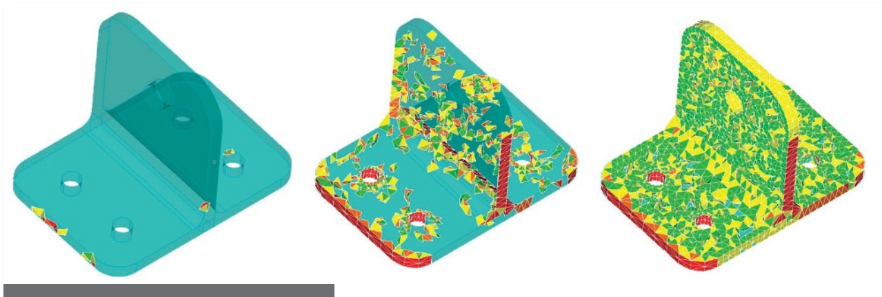
FIG. 6: A family of progressively distorted tetrahedral elements, with Jacobian checks.
